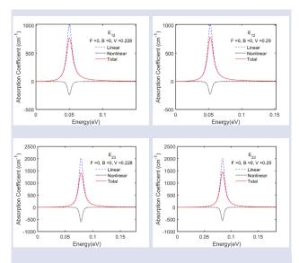
Figure 3. Absorption coeffients of the (1-2) and (2-3) transitions for different square quantum well barrier heights.
