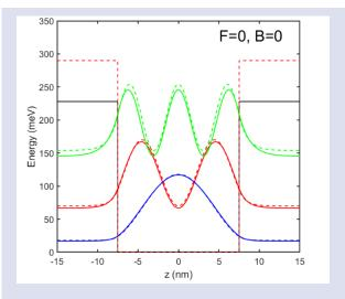
Figure 1. PDWs of first three energy states in the conduction band of QW structure in the for different quantum well barrier heights
